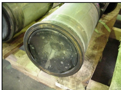
Deposits on Piston Crown
