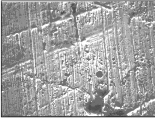
System wear caused by poor lubricity.
